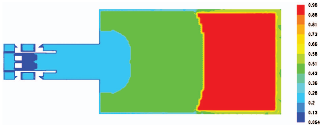
Fig. 3 Contour plot of grid cell size (mm). Cutting plane through center of combustor.
